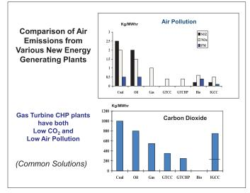
Figure 1. Gas-fired plants offer low emissions and high efficiency
