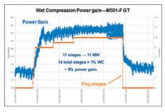
Wet Compression Power gain—M501-F GT: stages of wet compression were integrated with the Automatic Generation Control signal.
