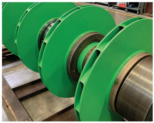
An anti-fouling coating applied to new impellers
