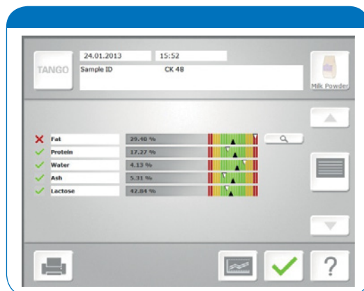
Figure 4: Result screen for a quantification showing a Mahalanobis outlier for the fat evaluation.
