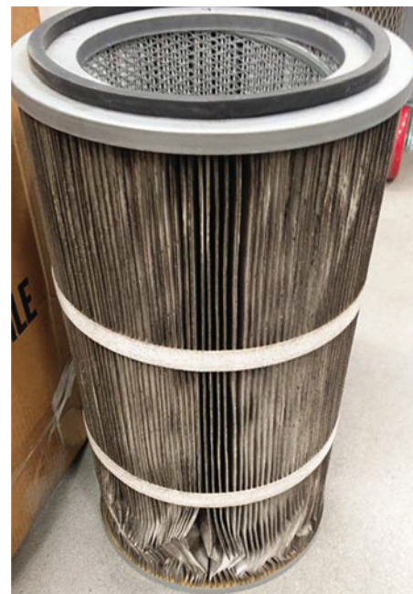
An inlet air filter with buckled pleats after three months due to the impact of water.
